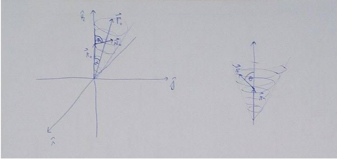
$$\vec{\Gamma}_z = m \vec{r}_0 \times \vec{v}_0 = -m z_0 v_0 \sin \Theta_0 \hat{i} = -\Gamma_z \hat{i}$$
