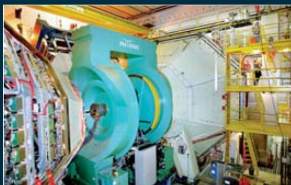
PHENIX experiment (shown here in partial disassembly during maintenance) searches for specific particles produced very early in the mini bangs.
