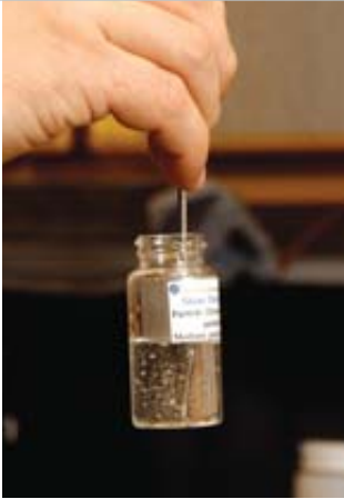
SHEAR-THICKENING FLUID stiffens instantly when an object is dragged through it, enabling a vial of the liquid to be lifted. It can improve Kevlar's bullet-stopping power.
