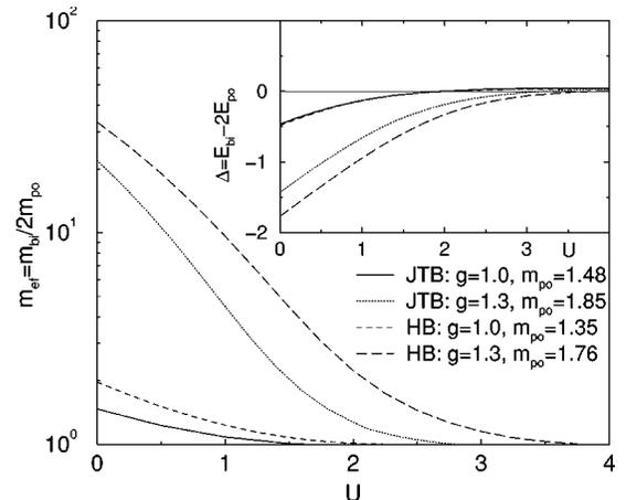
FIG. 10. Effective mass of JTB and HB results vs  $U$  for  $\omega_0=1.0$ . Inset: JTB and HB binding energies vs  $U$ . Finite-Hilbert space scaling was used for better accuracy.
