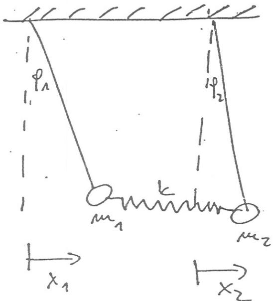
$$\begin{aligned}x_1 &= l \dot{\varphi}_1 & \ddot{x}_1 &= l \ddot{\varphi}_1 \\x_2 &= l \dot{\varphi}_2 & \ddot{x}_2 &= l \ddot{\varphi}_2\end{aligned}$$
