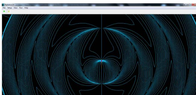
Figure 7. Dipole oscillation.
