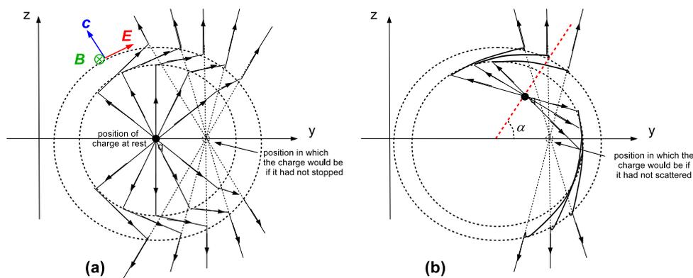
Figure 5. Field lines of an accelerated charge.
