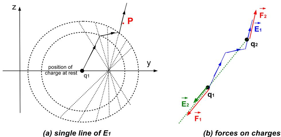
Figure 9. Electric field of accelerated charge and interaction forces.
