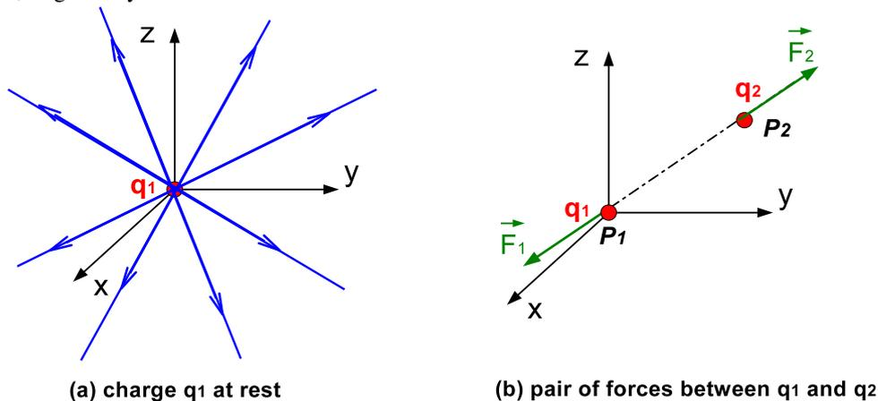
Figure 1. Field of charge at rest and electric forces.
