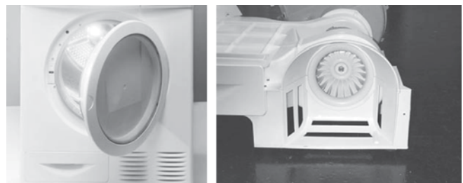
Fig. 3. Inlet channel to the secondary air-flow fan, basic version (left), modified versions I and II (right). The inlet slots on the front wall of the basic version were completely closed off and for modified versions I and II replaced with slots in the inlet duct so that the modified version drew all inlet air from the inside of the cabinet.
