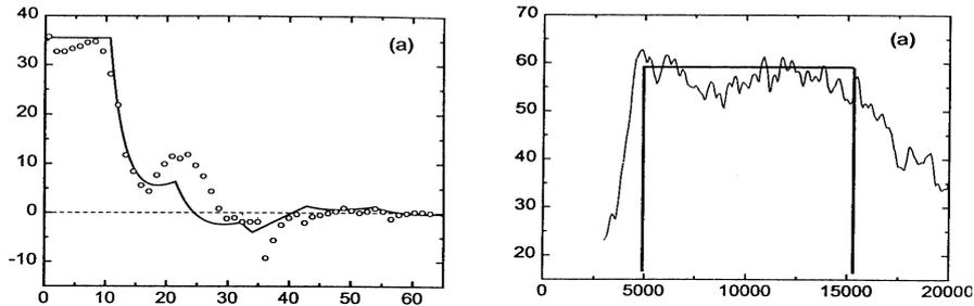
Fig. 16-17. Force between two parallel rigid plates as a function of the distance between them. The points are experimental data and the curves are from theory with no adjustable parameters for flat spectrum.
