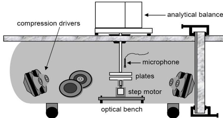
Fig. 12. The apparatus to measure the acoustic Casimir force
