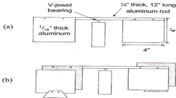
Fig. 13. The acoustic Casimir demonstration device
