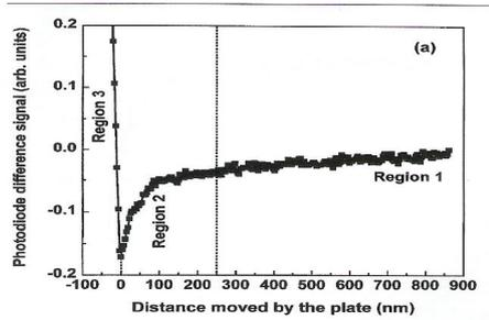
Fig. 9. A typical force curve as a function of the distance moved by the plate
