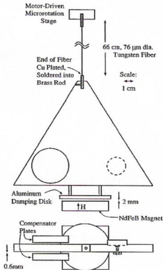
Fig.4. Details of the Lameroux pendulum. The body was total mass 397 g. The ends of the W fiber were plated with a Cu cyanide solution; the fiber ends were bent into hairpins of 1 cm length and then soldered into a 0.5 mm diam, 7 mm deep holes in the brass rods. Flat-head screws were glued to the backs of the plates; a spring and nut held the plates firmly against their supports end ensured good el. contact [7].
