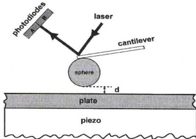
Fig. 7. Schematic diagram of experimental setup.
