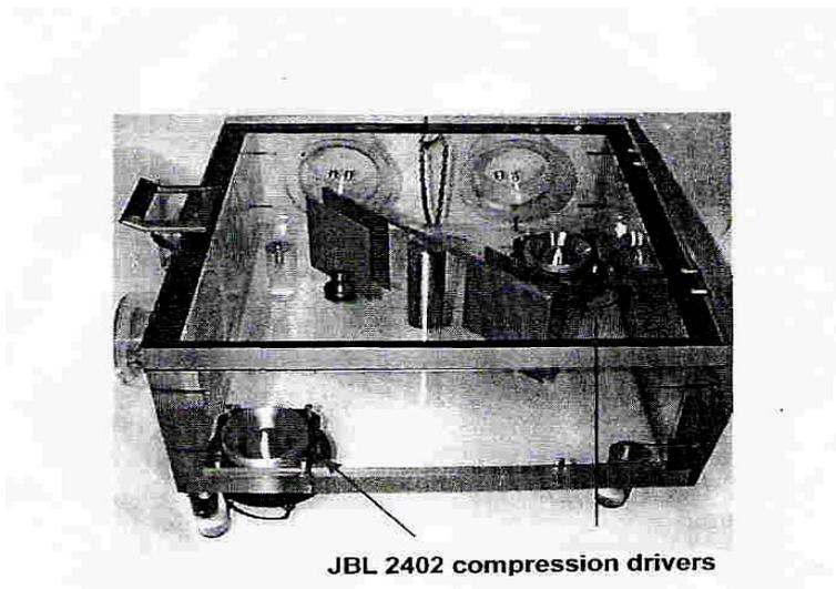
Fig. 14. The photograph of apparatus. The tank is made of 0,64 cm steel, length 1,5 m and diameter 0,5 m
