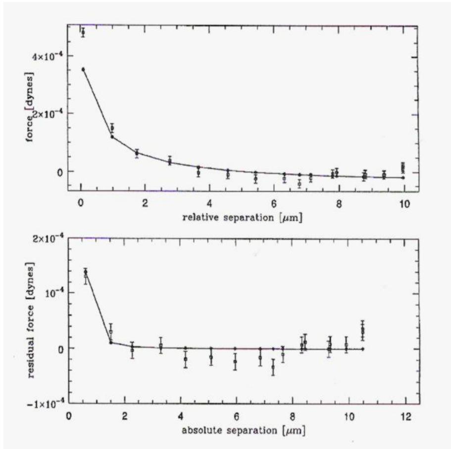
Fig.5-6. Top: Lameroux measured force as a function of relative position. Bottom: Measured force with electric contribution subtracted; the points connected by lines are as expected from the Casimir force [7].
