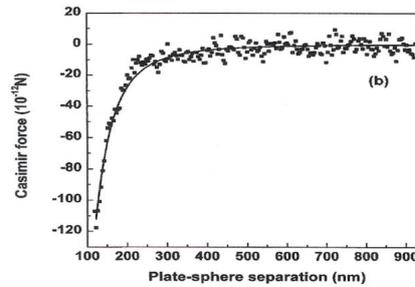
Fig. 10. The measured Casimir force as a function of sphere-plate surface separation.
