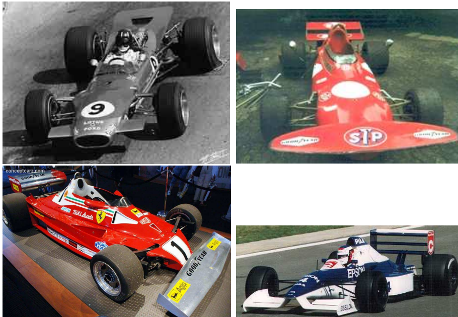
Figure 14: Some historical milestones in front wing development. Lotus 49B, March 711, Ferrari 312 T2 and Tyrrell 019.
