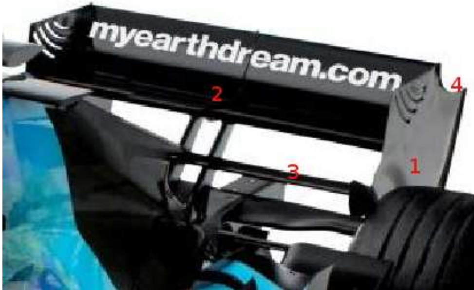
Figure 12: Modern rear wing consists of upper(2) an lower(3) airfoil section mounted on endplates (1) with U-shaped cutout (4).
