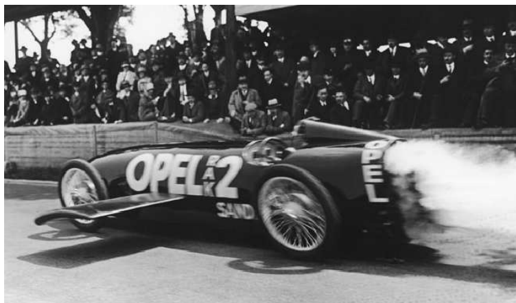
Figure 1: Opel's rocket powered RAK2, with large side wings
