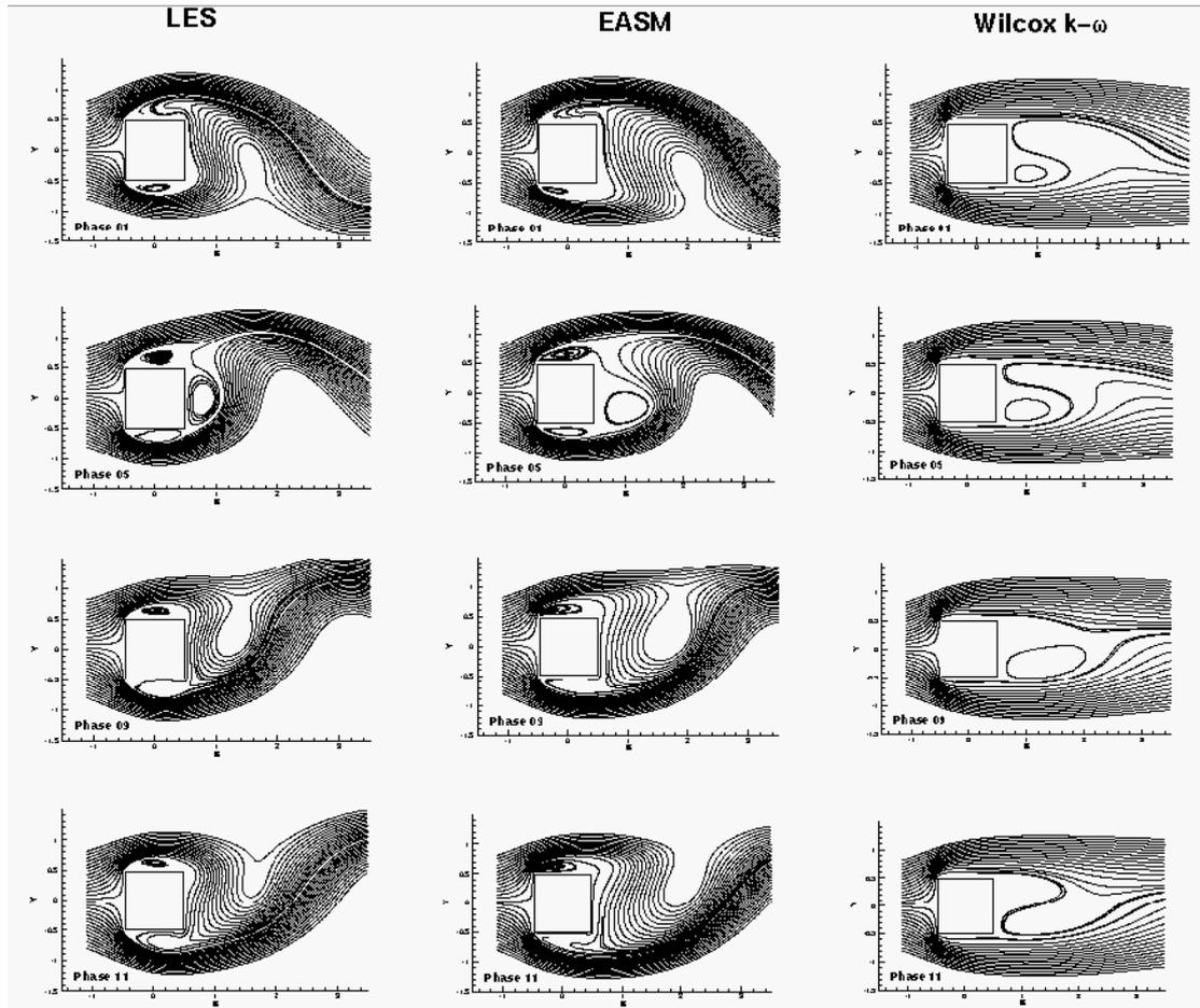
**Figure 5.2: Streamlines predicted by LES, EASM and RANS**
