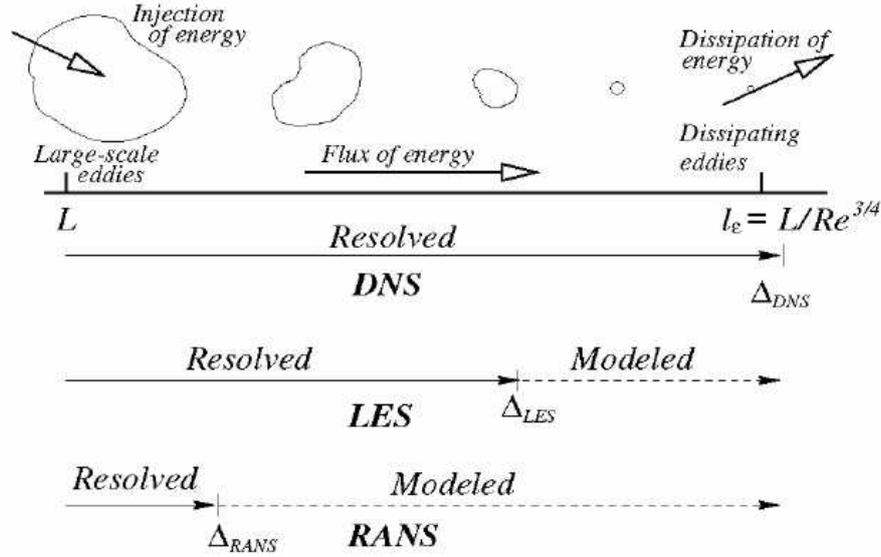
Figure 2.1 Extent of modelling for certain types of turbulent models
