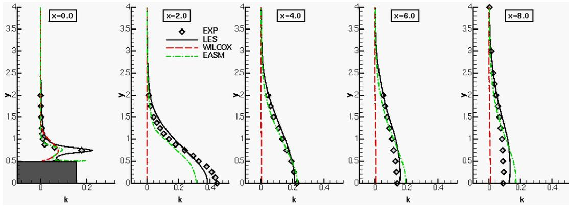
Figure 5.3: Turbulent kinetic energy in the wake region
