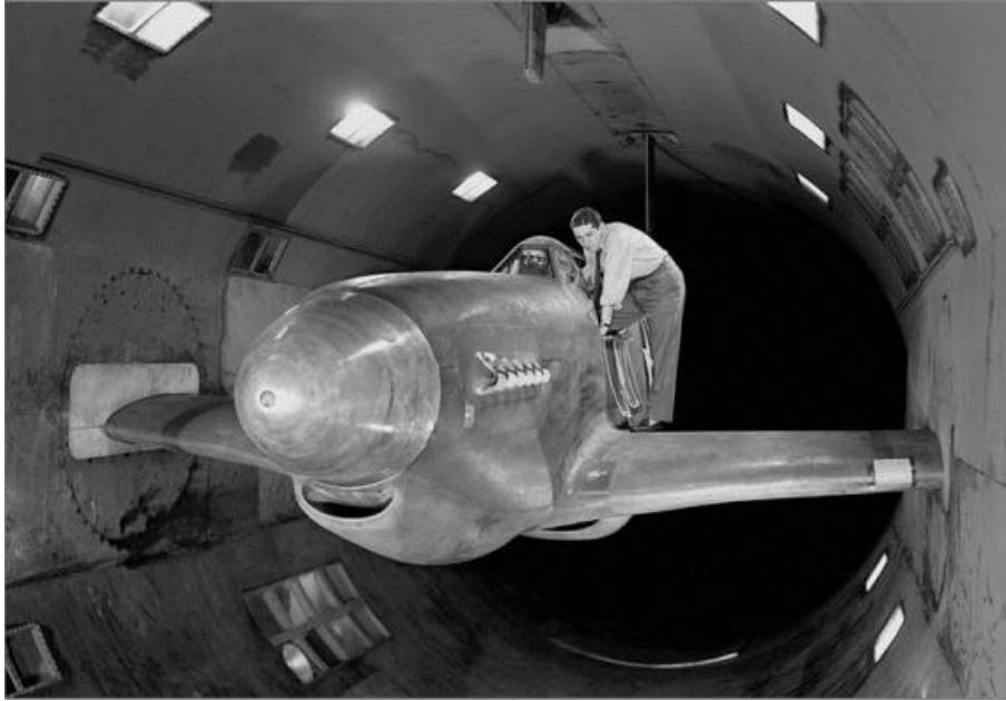
Image.6 The North American P-51 Mustang full scale model being tested in the NACA wind-tunnel.(NACA)
