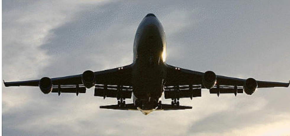
Image.7 Boeing 747 shows several sections of Fowler flaps during its final approach.
