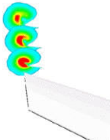
Image.3 The image above is the ONERA simulation of the wing-tip vortex separation.
