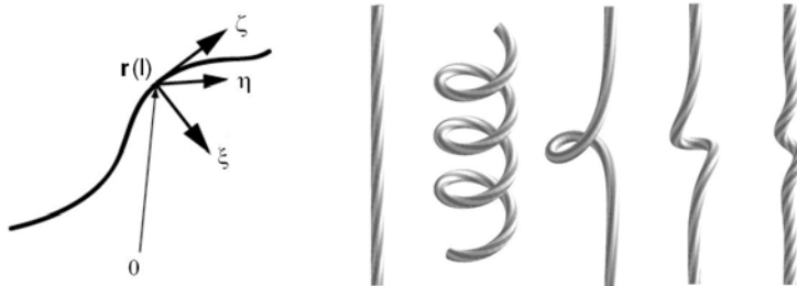
Figure 1: The \xi\eta\zeta frame moves along the length of the rod with unit velocity (left) [8]. The figure also shows selected solutions to Euler-Kirchhoff's equations that are important in the study of instability of elastic rods (right) [8].
