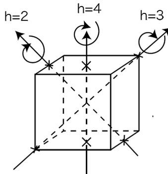
Figure 2: The symmetry axes of a cube
